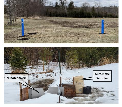
automatic water sampler which collects sequential water samples over time. Ausable Bayfield Conservation staff collect these samples which are then sent to a lab for analysis. At the field scale, surface runoff associated with
